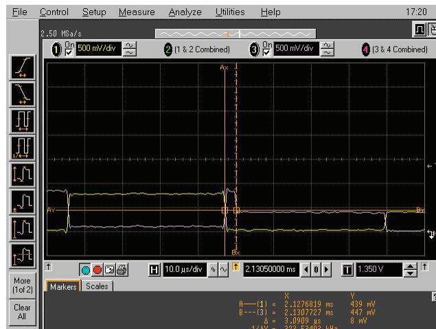
Figure 16. Time between last J in CHIRP and hi-speed termination initiation.
